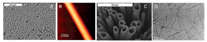
**Self-Assembled Nano-Structures:** (A) Scanning electron microscopy micrograph of peptide nanospheres. (B) Atomic force microscopy image of a peptide nanotube. (C) Array of ordered vertically aligned peptide nanotubes. (D) Transmittance electron microscopy micrograph of 3D hydrogel demonstrating the presence of elongated fibrils.
