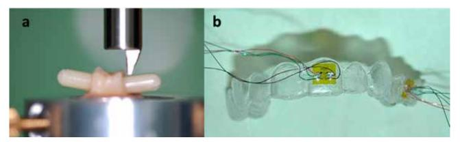
a. Shear bond test experiment. b. Transparent aligner equipped with strain gauges
