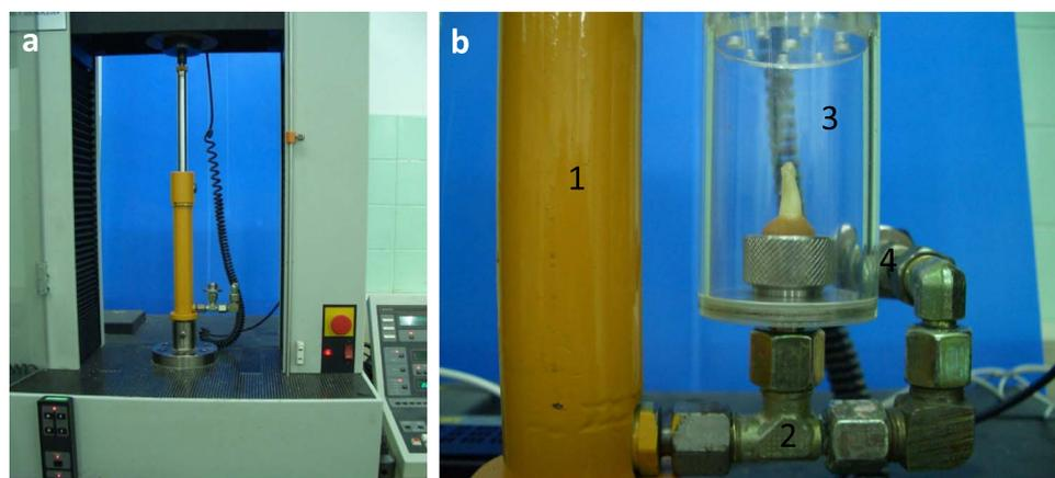
**Fig. 2.** Pressure generating system. (a) Piston filled with water connected to a universal loading machine. By loading the piston under compression, the pressure increased and the water was forced through the splitter into the external cannula that was bonded into the root canal. (b) Bursting chamber containing the mounted tooth. 1. Piston. 2. T-splitter. 3. Transparent bursting chamber. 4. Pressure transducer.
